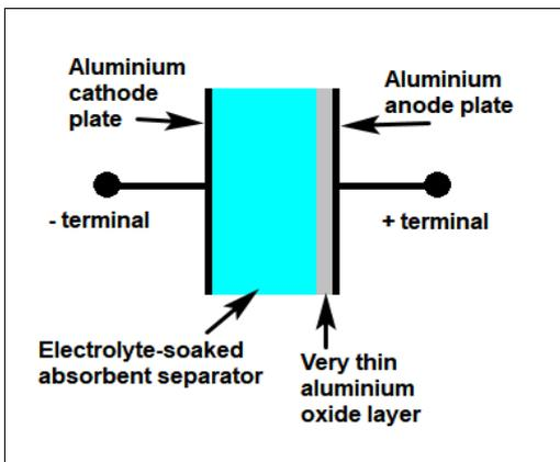
The electrolyte has some electrical resistance and it is between the cathode plate and the aluminium oxide dielectric so it's called the "Equivalent Series Resistance" or "ESR".
